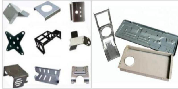
Punching, bending, shear cutting
