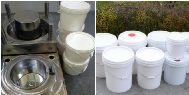
Bucket mold and bucket
