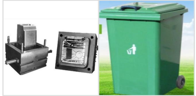
SMC mold and pressed SMC product
